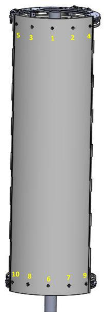
The panel is attached with 3/8-16 flat head Philips machine screws to the 90 degree brackets on the ring assemblies.
