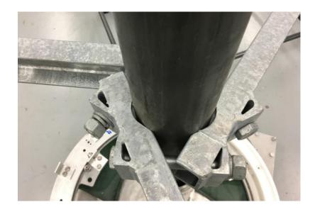
The three bolts should be tightened evenly to maintain 120 degree angular spacing between the three bars. Once the bolts are tightened the distance between the oval slots should be equal.
