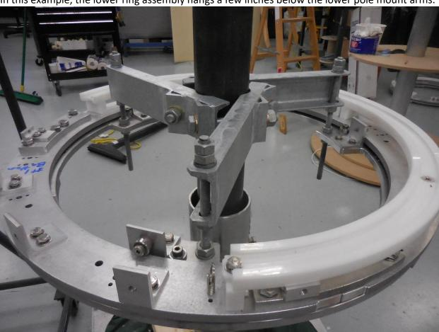
In this example, the lower ring assembly hangs a few inches below the lower pole mount arms.
